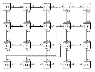
Fig 3: Two separate 9-node clusters can be made easily by switching some cables on the patch panel and disconnecting the two excess nodes. It is also possible to use 4x4 Cluster just by disconnecting 4 nodes (1, 4, 6, 11 or 20, 13, 15, 18).
