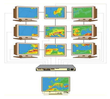
ig 1: Here we can see how parallel programming works on a 9-node cluster example. The domain of integration is divided into parts so every node calculates parameters on sub domains and after every time step they exchange the new values of variables. Standard Fortran code of the Eta model is modified using MPI (Message Passing Interface).
