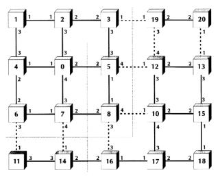
Fig 2: Here we can see how the 2-D grid looks on a 20 node cluster example. The domain of integration is divided in 20 parts, so every node calculates parameters on sub domain and after every time step they exchange new values of variables.
