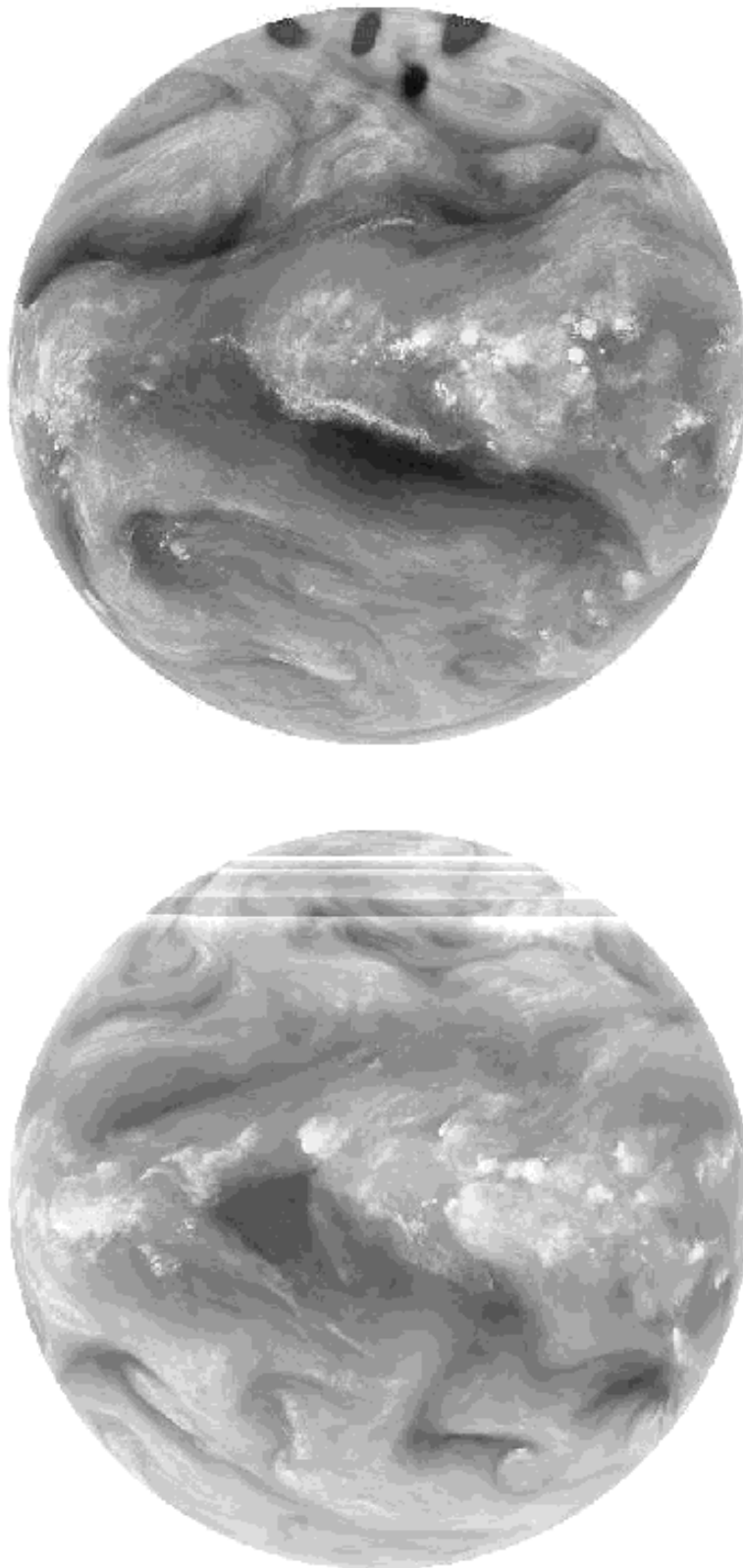
Figure 5: Top: Example of dark spots and bow shaped structures of anomalously high TB in a WV image at midnight. Bottom: Example of pattern of cold stripes at top of WV image. Images taken from EUMETSAT internet page http://www.eumetsat.de .
