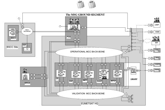
Fig. 1: The MSG Core Ground Segment.
