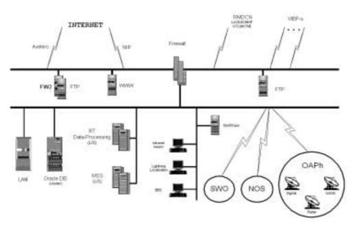
Fig. 1: HMS logical network diagram
