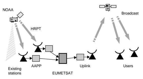
Fig. 3: The EUMETSAT ATOVS Retransmission Service (EARS) set-up.
