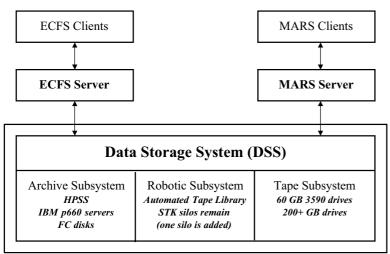
Figure 2 Structure of the Data Handling System
