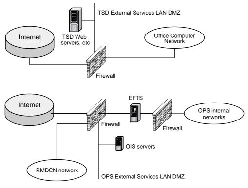
Fig. 2: The RMDCN set-up.
