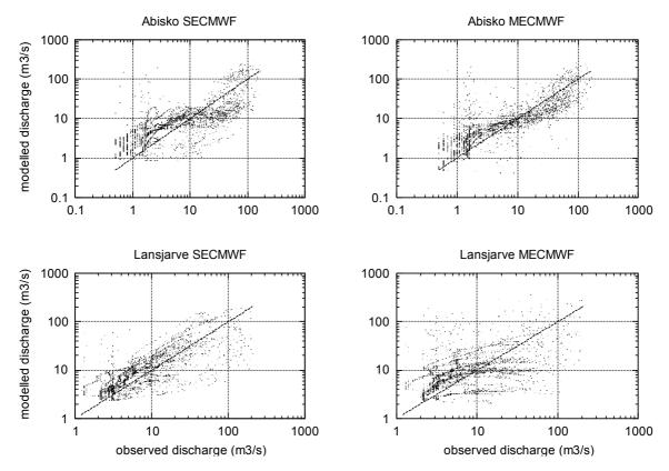
Figure 3: Scatterplot of daily observed and modelled discharge from the Abisko catchment (top panels) and Lansjärve catchment (bottom), for the model versions SECMWF (left) and MECMWF (right).
