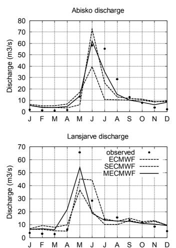
Figure 1: Simulated and observed discharge from the Abisko basin (top) and the Lansjärve calibration basin (bottom), averaged for 1989-1998.
