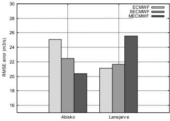
Figure 2: RMS error of daily discharge in the period 1989-1998 from the two subcatchments of Abisko and Lansjärve for each model version.
