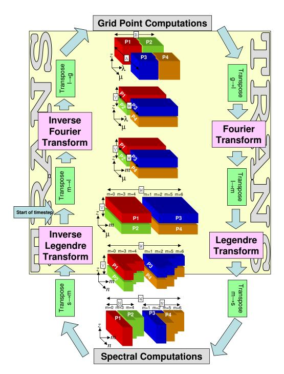
Figure 2.1: IFS Model Timestep, showing data decompositions
