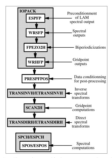
Figure E.10: Elements of  $\mathtt{STEPO}$  used for the post-processing. The greyish areas correspond to model subroutines.
