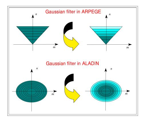
Figure D.3: Illustration of the gaussian spectral filter
