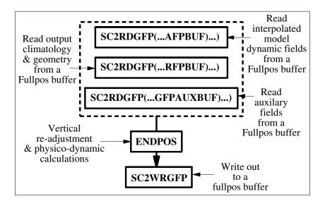
Figure E.14: Re-ajustements and physico-dynamic calculations on output grids : ENDVPOS.
