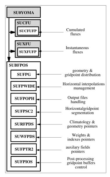
Figure E.4: Setup, second part : SUOYOMB. The greyish areas correspond to model subroutines.
