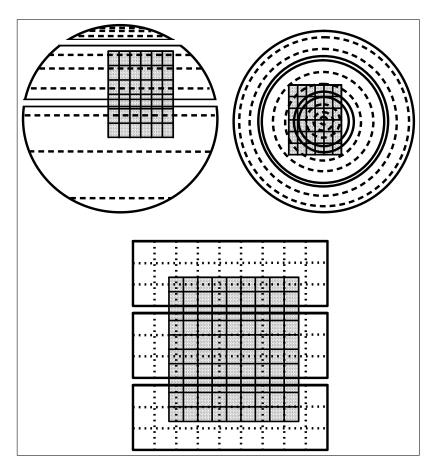
Figure E.18: Gridpoints repartitions betwen model and output grids: the greyish areas corresponds to an ouput grid; the background areas corresponds to the input model, with a physical separation between processors. Top left represents a typical coupling from a streched grid, Top right a typical coupling from a rotated grid, bottom a typical nesting.
