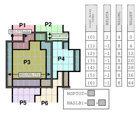
Figure 2.5: The semi-Lagrangian Halo (For processor 3)
