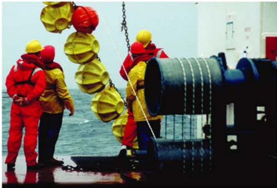
Sense of urgency: scientists on the Discovery deploy moorings that carry sensors to the ocean floor.
