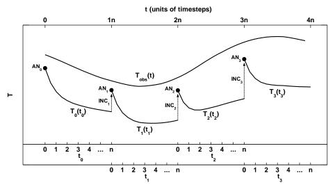
Schematic diagram showing the data assimilation / forecast cycle
