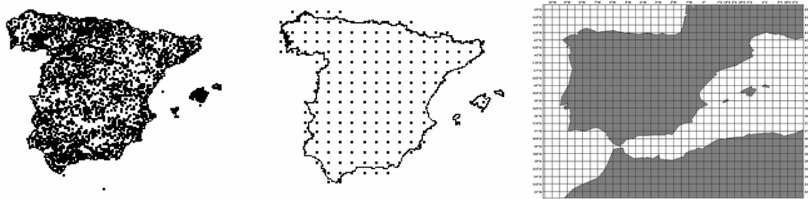
Figure 3: From left to right, pluviometric network, 203-point mesh and 0.5° grid resolutions of the regional RCA model over the Iberian peninsula, respectively.
