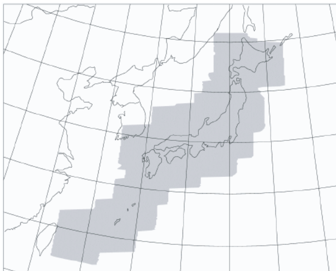
Fig. 1. The forecast domain of JMA Meso-Scale Model. The radar-AMeDAS precipitation analysis data are available within the gray area.
