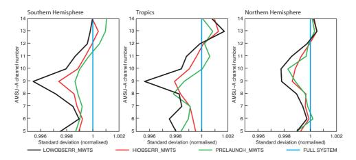
Figure 2: Normalised standard deviations of first guess departures for AMSU-A channels 5-14, aggregated over all actively assimilated AMSU-A's during the period 1 May 2010 - 30 July 2010. The normalisation is with respect to the standard deviations for the FULL SYSTEM OSE.
