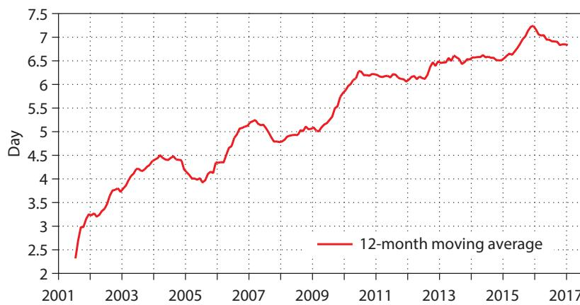
**Figure 8** Time evolution of the forecast lead time when the CRPSS for the prediction of 24-hour accumulated precipitation drops below 0.1. Forecasts are verified against observations at SYNOP network weather stations in the extratropics.
