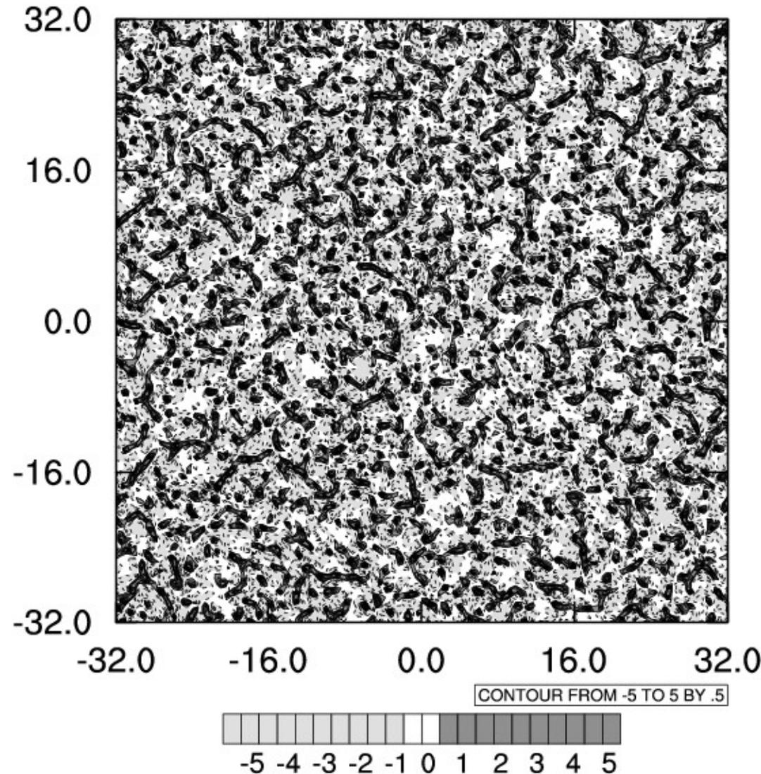
Convection over heated plane, heatflux  $.2 \text{ Kms}^{-1}$ ,
